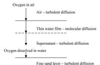
Figure 6-2 Oxygen diffusion pathway in a single sand layer BSF
