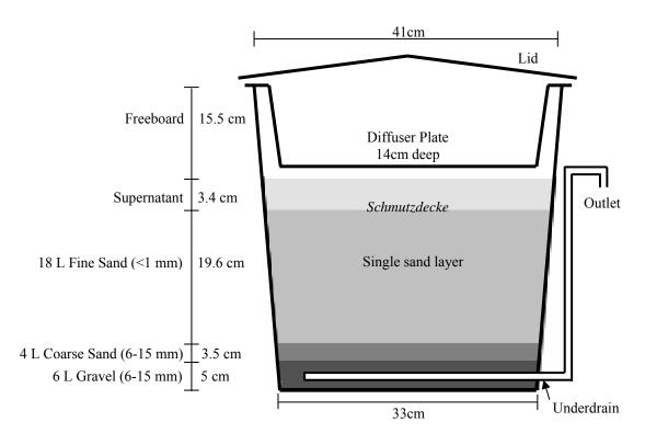
Figure 6-4 Single sand layer biosand filter (BSF A)
