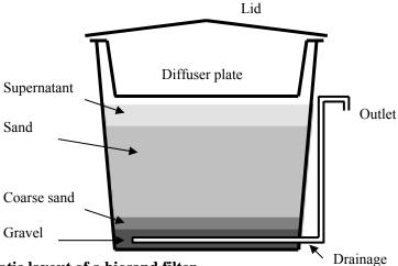
Figure 3-2 Schematic layout of a biosand filter
