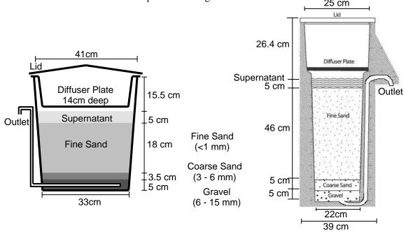
Figure 5-4 Single sand layer biosand filters: a) local plastic design and b) concrete design (Source: concrete filter from CAWST 2009b)
