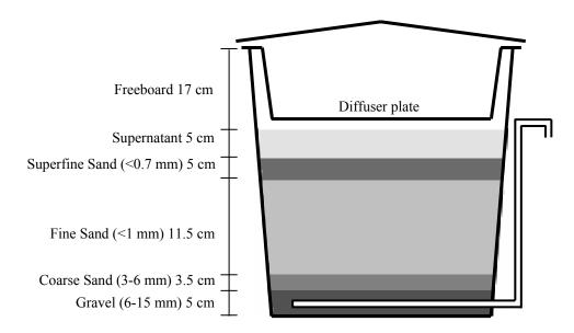
Figure 5-2 Biosand filter with superfine sand layer
