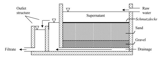
Figure 3-1 Schematic layout of a slow sand filter
