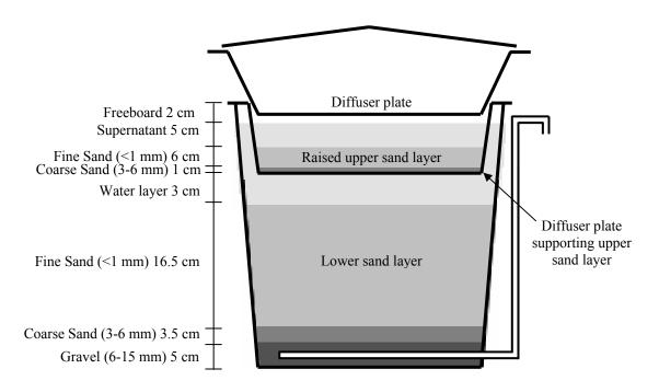
Figure 5-3 Biosand filter with dual sand layers
