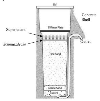
Figure 3-4 CAWST style BSF filter layout
