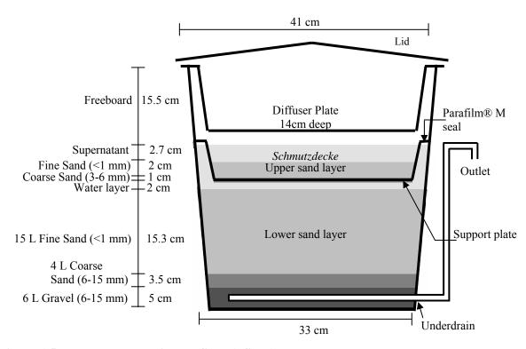
Figure 6-5 Dual sand layer biosand filter (BSF B)
